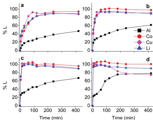
**Fig. 1** Leaching efficiencies (%L) of LiCoO<sub>2</sub> + Al + Cu mixtures in choline chloride–citric acid DES as a function of time at different temperatures. Temperatures: room temperature (left above, a), 40 °C (right above, b), 60 °C (left below, c) and 80 °C (right below, d). DES: ChCl : CA 2 : 1 +35 wt% H<sub>2</sub>O. Leaching parameters: S : L = 20 g L<sup>-1</sup>, Al : LiCoO<sub>2</sub> = 12 wt%, Cu : LiCoO<sub>2</sub> = 24 wt% at 900 rpm.
