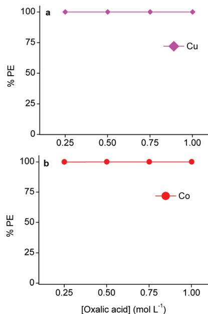
**Fig. 9** Efficiencies of stripping precipitation of metal oxalates at different oxalic acid concentrations. (a) Cu(i/ii) oxalate formation by stripping from loaded 60 vol% LIX 984 in an aliphatic diluent and (b) cobalt(ii) oxalate formation by stripping from loaded undiluted water-saturated A336. The loaded LIX 984 and A336 contained 4.7 g L<sup>-1</sup> Cu(i/ii) and 9.8 g L<sup>-1</sup> Co(ii). Phase ratio = 1:1, equilibration = 30 min, shaking speed = 2250 rpm, room temperature.
