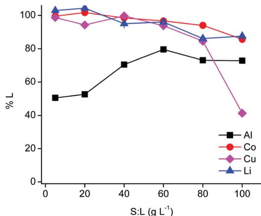
**Fig. 2** Variation of the solid-to-liquid ratio (S:L) during leaching by choline chloride–citric acid DES. Composition of the DES: ChCl : CA 2 : 1 +35 wt% H<sub>2</sub>O. Leaching parameters: 1 h at 40 °C, Al : LiCoO<sub>2</sub> = 12 wt%, Cu : LiCoO<sub>2</sub> = 24 wt% at 900 rpm.
