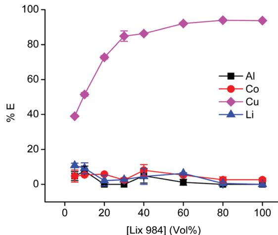
Fig. 8 Optimisation of the LIX 984 concentration in the aliphatic diluent during extraction of metals from the PLS. Initial metal concentrations in the PLS: Al(III)  $1.0 \text{ g L}^{-1}$ , Co(II)  $12.1 \text{ g L}^{-1}$ , Cu(I/II)  $4.7 \text{ g L}^{-1}$  and Li (I)  $1.1 \text{ g L}^{-1}$ . Equal phase ratio was used. Equilibration time = 30 min, shaking speed = 2250 rpm, room temperature.
