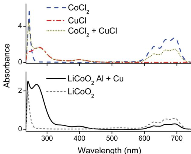
**Fig. 5** Optical absorption spectra of the DES pregnant leach solution. DES: ChCl:CA 2:1 +35 wt% H<sub>2</sub>O. Input concentrations CuCl, CoCl<sub>2</sub> ca. 2 g L<sup>-1</sup>, the PLS was diluted 40 times. Metal chloride salts (above) compared with the spectra of the PLS (below) with and without the Al and Cu.
