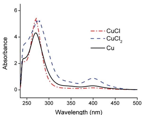
**Fig. 4** Optical absorption spectra of CuCl (red curve) and CuCl<sub>2</sub> (blue curve) dissolved in the choline chloride–citric acid DES. The black lines is the absorption spectrum of the copper species formed by dissolution of copper metal in the DES. DES: ChCl:CA 2:1 +35 wt% H<sub>2</sub>O. Concentrations of the dissolved copper ions in the DES are ca. 1 g L<sup>-1</sup>.
