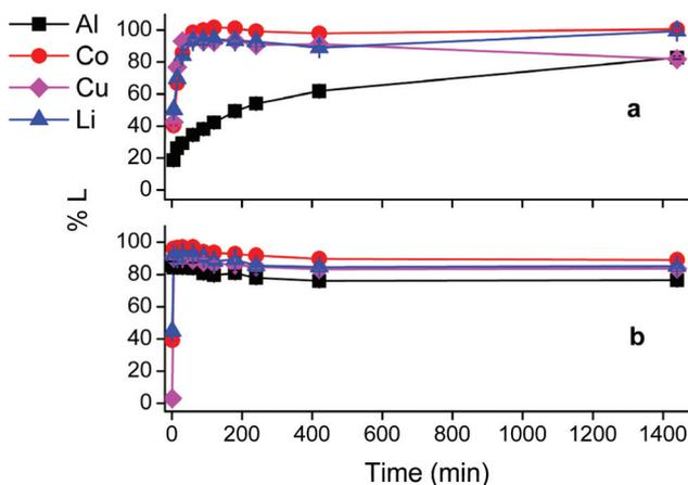
**Fig. 6** Comparison between leaching with leaching of  $\text{LiCoO}_2$  by DES and HCl solution. Top: DES leaching ( $\text{ChCl}:\text{CA } 2:1 + 35 \text{ wt\% H}_2\text{O}$ ). Bottom: Leaching with HCl  $1 \text{ mol L}^{-1}$ . Leaching parameters: S:L = 20 g  $\text{L}^{-1}$ , 40 °C, Al:  $\text{LiCoO}_2 = 12 \text{ wt\%}$ , Cu:  $\text{LiCoO}_2 = 24 \text{ wt\%}$  at a stirring rate of 900 rpm.
