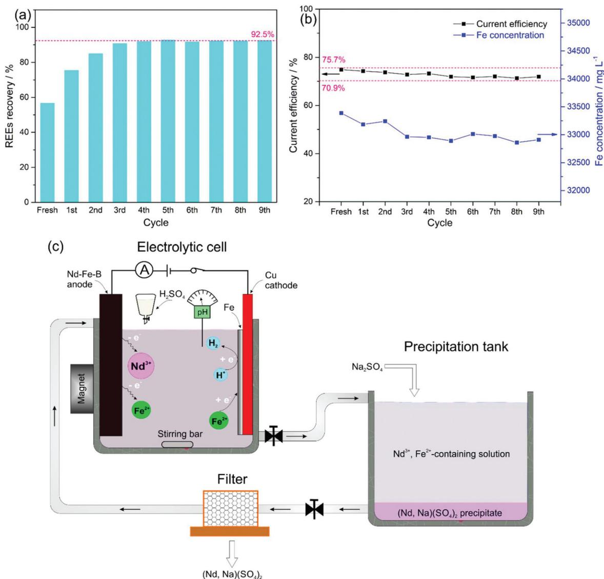
Fig. 4 (a) Percentage extraction of REEs at an anodic current density of  $25 \text{ mA cm}^{-2}$  and a cathodic current density of  $12.5 \text{ mA cm}^{-2}$  and (b) current efficiency of Fe deposition and total dissolved Fe concentration over 9 recycling cycles. (c) Schematic of the proposed closed-loop recycling route for recovering REEs from the sintered Nd–Fe–B magnets.
