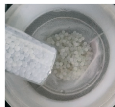
Fig. 8 Colour difference between pristine, unused beads, and those which had been used in testing multiple times.
