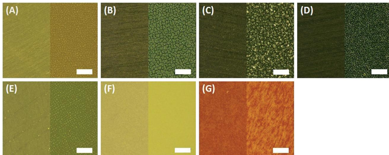
**Fig. 2** Optical images (250 $\times$ ) of surfaces of: (A) unfilled epoxy, (B) epoxy-carbon black composite, (C) epoxy-graphene composite, (D) epoxy-MWCNT composite, (E) epoxy-SiO<sub>2</sub> composite, (F) unfilled polypropylene, (G) PP-Fe<sub>2</sub>O<sub>3</sub>. The left half of each image shows un-weathered sample and the right half shows samples weathered for 2500 h in an accelerated wet weathering chamber. Scale bar is 250  $\mu$ m for all images.
