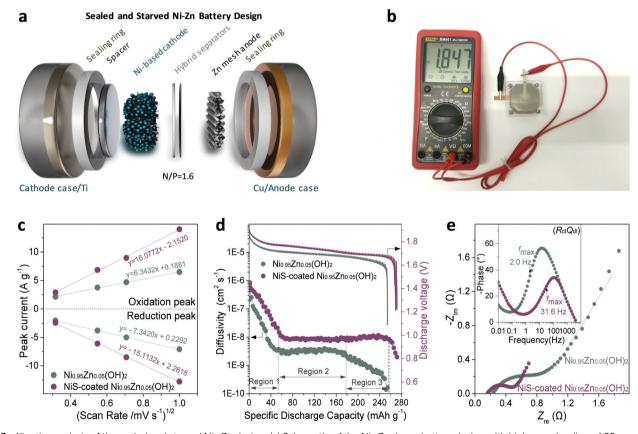
Fig. 3 Kinetics analysis of the sealed and starved Ni–Zn design. (a) Schematic of the Ni–Zn demo battery design with high mass loading of 80 mg cm<sup>-2</sup>. (b) Photograph of the designed cell and high open-circuit voltage of 1.847 V of the Ni-Zn cell. (c) Linear correlation between the peak current and the square root of the scan rate. (d) GITT curves and diffusivity versus DOD. (e) Nyquist plots. Inset: Bode plots of the (RctOdi) parallel components.
