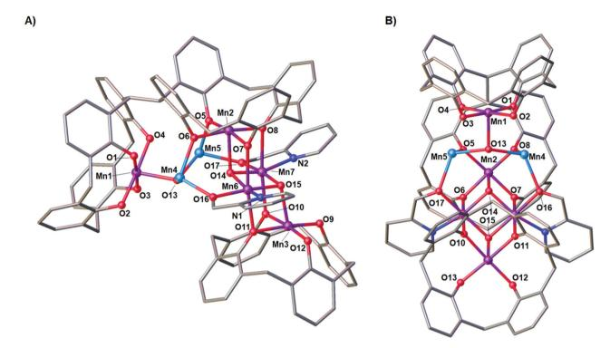
Fig. 3 Side (A) and orthogonal (B) views of the partial single crystal X-ray structure of the asymmetric unit in 6. Selected labels have been added according to discussion. Colour code C – grey, O – red, N – royal blue,  $Mn^{II}$  – pale blue,  $Mn^{III}$  – purple. Hydrogen atoms, <sup>t</sup>Bu groups, ligated solvent molecules and co-crystallised solvent/anions omitted for clarity. Figures not to scale.
