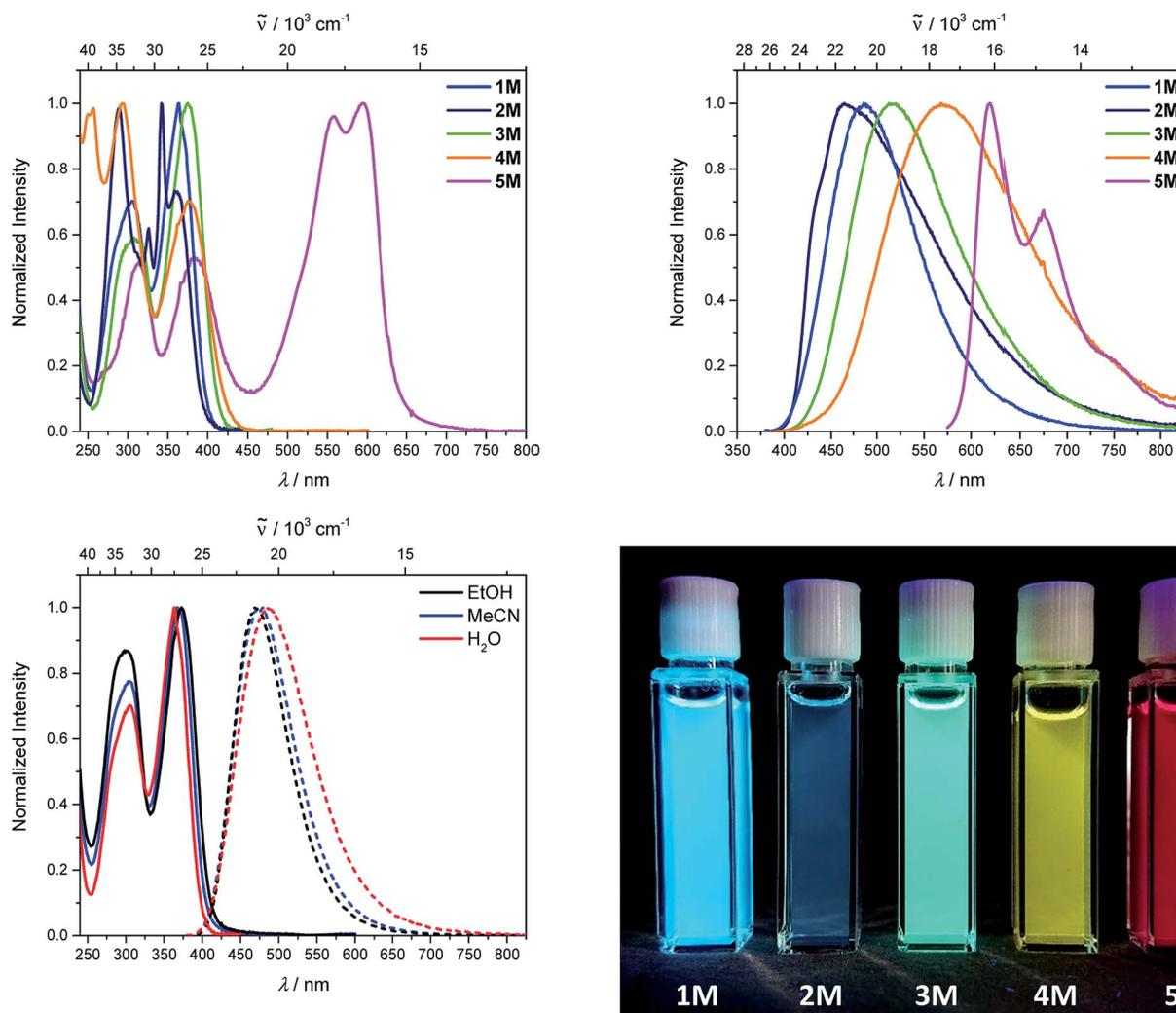
Fig. 3 Absorption (top, left) and emission spectra (top, right) of **1M**–**5M** in water. Compound **2M** was dissolved in 10% MeCN in water. Absorption and emission spectra of **1M** in various solvents (EtOH: black, MeCN: blue, H<sub>2</sub>O: red) (bottom, left) and picture of the solutions of **1M**–**5M** in MeCN under UV irradiation.
