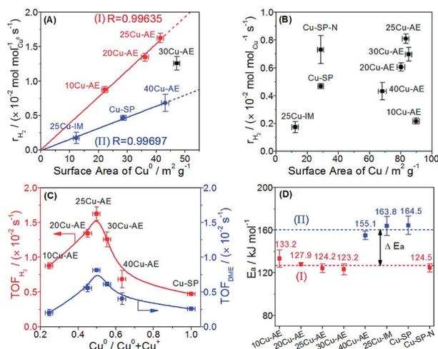
Fig. 4 Correlation of the H<sub>2</sub> production rate based on Cu<sup>0</sup> sites or total Cu sites with (A) the surface area of Cu<sup>0</sup> and (B) total surface area of Cu; (C) correlation of the TOF of H<sub>2</sub> and DME with the Cu<sup>0</sup>/(Cu<sup>0</sup> + Cu<sup>+</sup>) ratio; (D) apparent activation energies of the catalysts.
