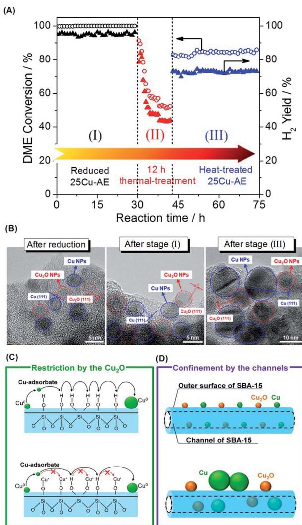
Fig. 3 (A) Stabilities of 25Cu-AE upon thermal treatment. Reaction conditions: (I) and (III): GHSV = 18 000 h<sup>-1</sup>, S/C = 2/1 (mol mol<sup>-1</sup>), T = 400 °C; (II): GHSV = 36 000 h<sup>-1</sup>, S/C = 2/1 (mol mol<sup>-1</sup>), T = 450 °C; (B) TEM images of 25Cu-AE during the stability test; (C) schematic representation of the restriction by the adjacent Cu<sub>2</sub>O; (D) schematic illustration of the spatial confinement by the channels.
