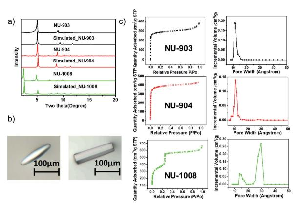
Fig. 3 Characterization of the three MOFs. (a) PXRD patterns; (b) optical images of the single crystals of NU-904 (left) and NU-1008 (right), the scale bars in the images are 100  $\mu$ m; (c) N<sub>2</sub> sorption isotherms and DFT pore size distribution of NU-903, NU-904 and NU-1008.
