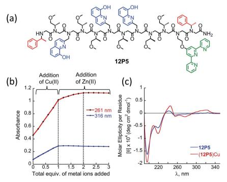
Fig. 8 (a) Chemical sequence of the peptoid oligomer 12P5. (b) A plot representing absorbance at 261 nm and 316 nm as a function of total equivalents of metal ions added from the UV-Vis titration of 12P5 with first 1 equiv.  $Cu^{2+}$  followed by addition of  $Zn^{2+}$ , at the concentration of 17 μM in 4 : 1 MeOH :  $H_2O$  solution. (c) CD spectra of the peptoid 12P5 and (12P5)Cu complex, at the concentration of 100 μM in 4 : 1 MeOH :  $H_2O$  solution.
