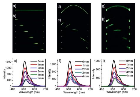
Fig. 5 Phosphorescent optical waveguide properties of single DBBZL crystals in straight shape (a-c), in elastic bent shape (d-f) and in plastic bent shape (q-i). Photographs of the crystal under UV light (a, d and g); images collected at different positions of the crystal upon 355 nm laser (b, e and h). Phosphorescent spectra measured at one end of the crystal with constantly changing distances between the end and the laser excitation positions (c, f and i).
