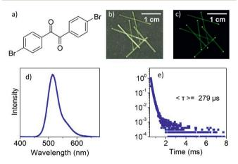
Fig. 1 Molecular structure of DBBZL (a); photographs of single DBBZL crystals taken under daylight (b) and 365 nm UV light (c); emission spectrum of the DBBZL crystal (d); phosphorescent decay curve of DBBZL measured at 514 nm (e).
