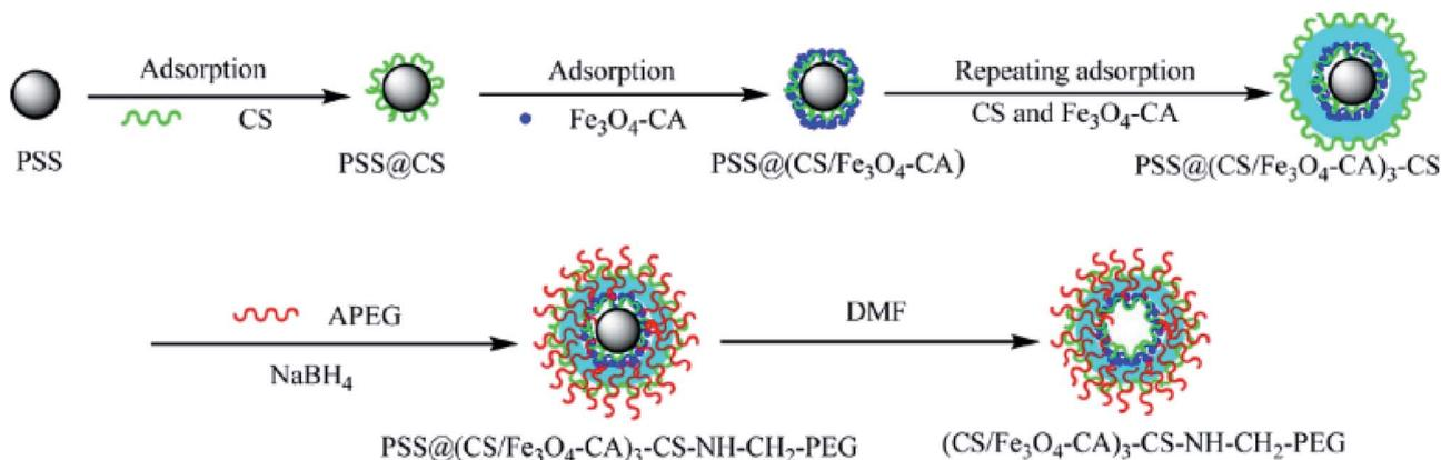
Fig. 3 Schematic of the preparation of superparamagnetic polyelectrolyte hybrid hollow microspheres.<sup>57</sup>
