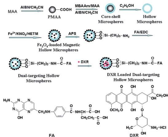
Fig. 11 Preparation of magnetite and tumor dual-targeting P(MBAAm-*co*-MAA) hollow microspheres as anticancer drug-carriers and the chemical structures of FA and DXR molecules.<sup>90</sup>
