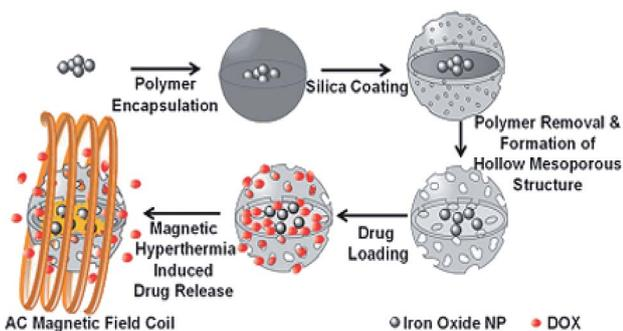
Scheme 4 Schematic of the preparation and drug loading of the porous hollow Fe<sub>3</sub>O<sub>4</sub>@C nanocapsules.<sup>79</sup>
