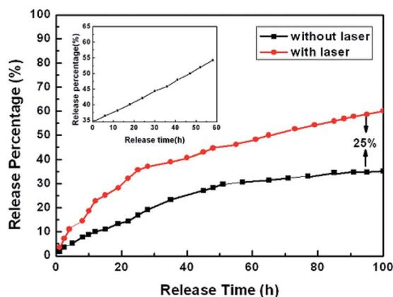
Fig. 9 *In vitro* release profiles of DOX-Au@Fe<sub>3</sub>O<sub>4</sub>@C nanoparticles with (red) and without (black) laser irradiation for 100 h. Inset: further DOX release (black) on the balance for another 60 h with laser radiation.<sup>80</sup>
