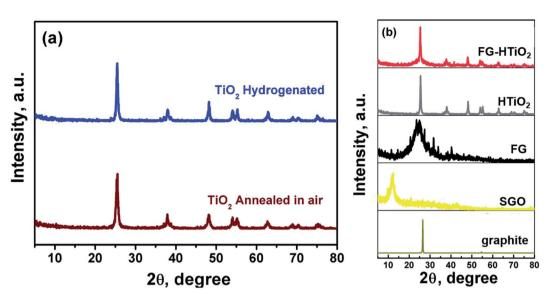
Fig. 2 XRD patterns of (a) air- and H<sub>2</sub>-annealed TiO<sub>2</sub>, and (b) pristine graphite, SGO, FG, HTIO<sub>2</sub> and FG-HTiO<sub>2</sub>.
