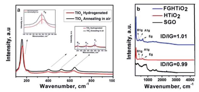
Fig. 4 Raman spectra of (a) air- and H<sub>2</sub>-annealed TiO<sub>2</sub>, and (b) pristine graphite, SGO, FG, HTIO<sub>2</sub> and FG-HTiO<sub>2</sub>.
