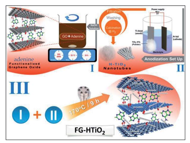
Scheme 1 Stepwise preparation of FG-HTiO<sub>2</sub>.
