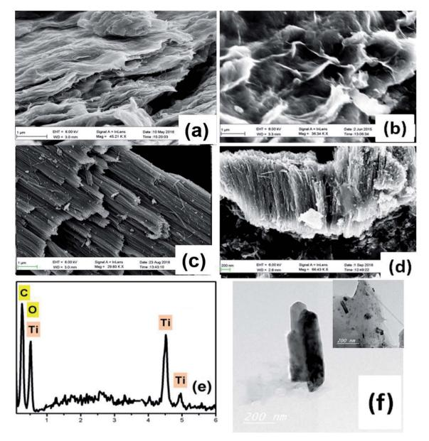
Fig. 1 FESEM images of (a) spongy GO, (b) FGO, (c) HTiO<sub>2</sub>, (d) FG-HTiO<sub>2</sub>, (e) EDS image and, (f) the TEM image of FG-HTiO<sub>2</sub> of the functionalize graphene-hydrogenated TiO<sub>2</sub> hybrid nanostructure.
