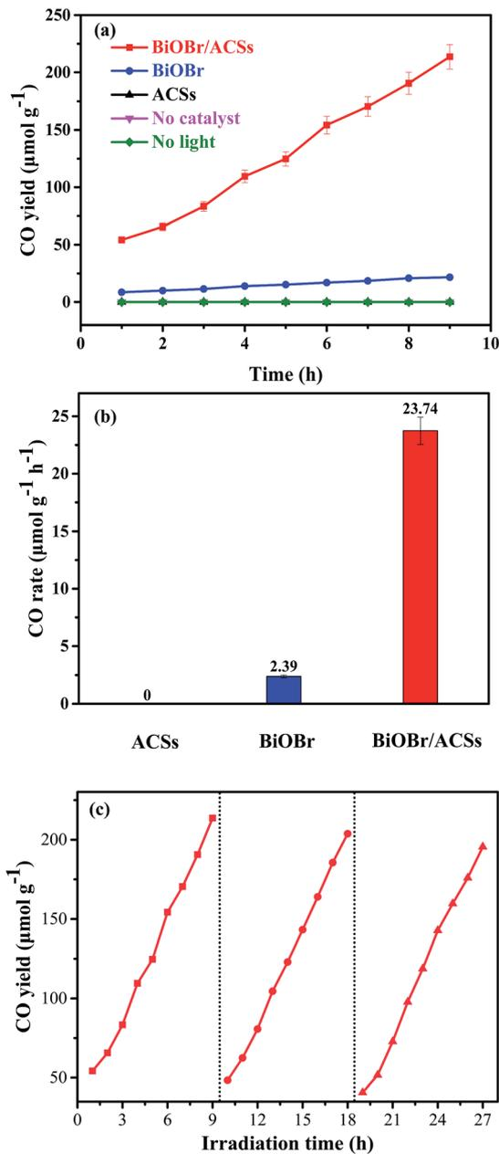
Fig. 6 Photocatalytic CO<sub>2</sub> reduction over BiOBr and BiOBr/ACSS samples under UV-vis irradiation: (a) CO yield, (b) CO rate and (c) cyclic experiments.
