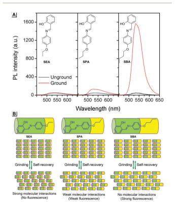
Fig. 4 (A) Fluorescence spectra of **SEA**, **SPA** and **SBA** before and after grinding. (B) Proposed mechanism for the fluorescence changes.
