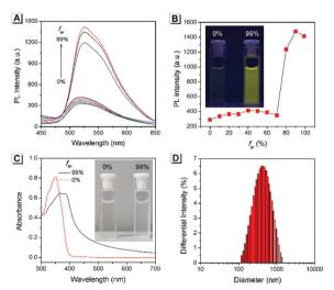
Fig. 1 (A) Fluorescence spectra of SBA in water/ethanol mixtures with different  $f_{\rm w}$ . (B) Fluorescence intensity of **SBA** at 525 nm as a function of  $f_{\rm w}$ . (C) Absorption spectra of **SBA** in water/ethanol mixtures with  $f_w$  of 0% and 99%. (D) DLS result of **SBA** in water/ethanol mixtures with an  $f_{\rm w}$  of 99%. Inset: A photo of **SBA** in water/ethanol mixtures with  $f_w$  of 0% and 99%; (B) under UV light irradiation and (C) under daylight.
