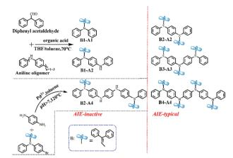
Scheme 1 Synthesis of oligoaniline derivatives substituted with diphenyl enamines
