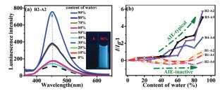
Fig. 3 (a) Emission spectra of B2-A2 in THF/water mixtures under excitation at 335 nm (10 µM; EX slit: 5 nm; EM slit: 10 nm). Inset: Fluorescent images of B2-A2 in THF/water mixtures containing 0 and 90% water. (b) Plots of  $(I/I_0) - 1$  vs. water content for six aniline derivatives, where  $I_0$  is the luminescence intensity in pure THF.
