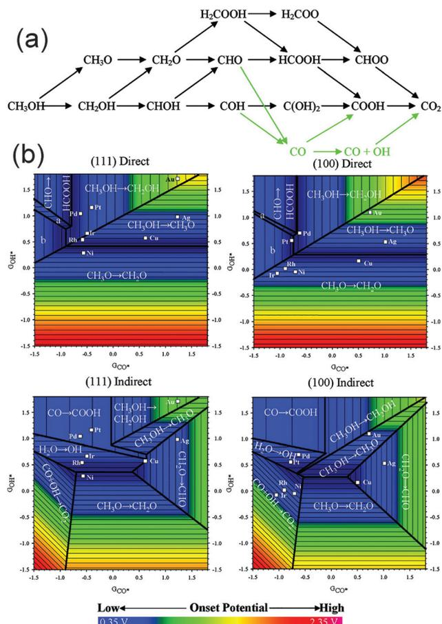
**Fig. 16** (a) Schematic representation of the reaction pathways and possible intermediates considered here for methanol electrooxidation. Green arrows indicate the indirect mechanism to  $\text{CO}_2$  formation. (b) Potential-determining steps for methanol electrooxidation on (111) and (100) facets plotted using  $G_{\text{CO}^+}$  and  $G_{\text{OH}^+}$  as the descriptors. Adapted with permission from ref. 190. Copyright 2009, American Chemical Society.
