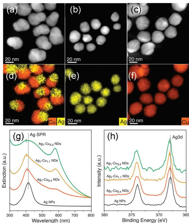
**Fig. 25** (a–c) HAADF-STEM images of Ag<sub>1</sub>-Cu<sub>1.1</sub> NDs (a), Ag NPs (b), and Cu NPs (c); (d–f) corresponding EDX elemental maps of Cu (orange) and Ag (yellow) of Ag<sub>1</sub>-Cu<sub>1.1</sub> NDs (d), Ag NPs (e), and Cu NPs (f). (g) UV-vis spectra and (h) XPS spectra of Ag/Cu nanocrystals. Adapted with permission from ref. 279. Copyright 2019, American Chemical Society.
