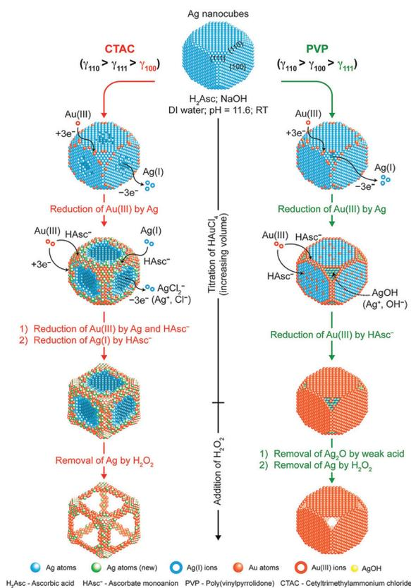
**Fig. 7** Schematic illustration describing the mechanisms proposed for the deposition of Au and Ag atoms on Ag NCs when  $\text{HAuCl}_4$  is titrated into an aqueous suspension of Ag NCs in the presence of  $\text{H}_2\text{Asc}$ ,  $\text{NaOH}$ , and CTAC (left) or PVP (right) at an initial pH of 11.6. Adapted with permission from ref. 101. Copyright 2017, American Chemical Society.
