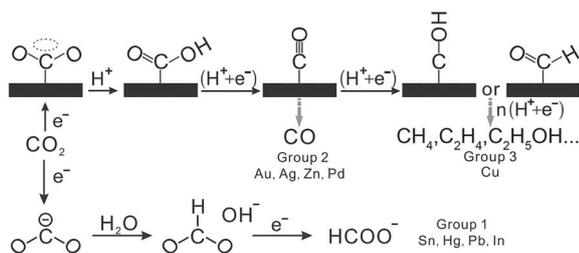
**Fig. 24** Reaction mechanism of electrochemical CO<sub>2</sub>RR on metal electrodes in aqueous solutions. Adapted with permission from ref. 271. Copyright 2016, Wiley-VCH.
