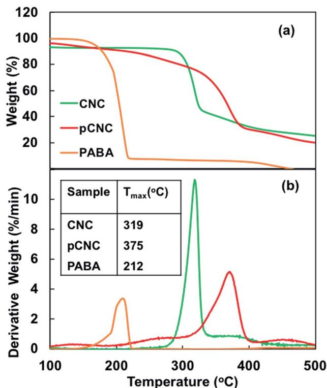
Fig. 3 TGA analysis of CNCs, PABA and pCNC: (a) weight loss curve and (b) weight loss derivative curve.
