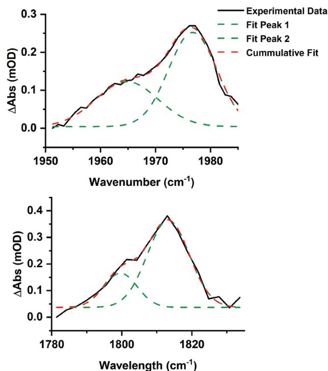
Fig. 4 Gaussian deconvolution of the bands at in the region 1950–1990 cm<sup>-1</sup> (top,  $R^2 = 0.986$ ) and 1780–1830 cm<sup>-1</sup> (bottom,  $R^2 = 0.970$ ) at 10 ps. Parameters are listed in Table 1.
