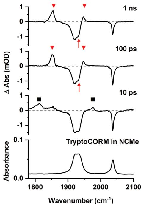
Fig. 3 Bottom IR spectrum of trypto-CORM in NCMe in the region 1780–2100 cm<sup>-1</sup>. Top time-resolved difference IR spectra for the photolysis (400 nm) of trypto-CORM in NCMe with pump-probe delays of 10 ps, 100 ps, and 1 ns showing bands for A and B (■) and C by (▼). The red arrows show the apparent recovery of the GSB for trypto-CORM.
