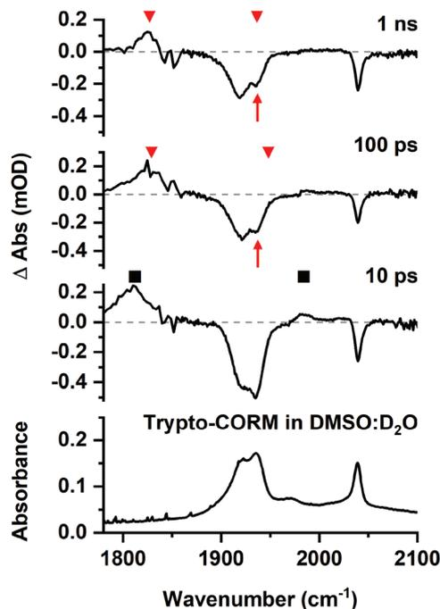
**Fig. 8** Bottom IR spectrum of trypto-CORM in DMSO:D<sub>2</sub>O (1:9 v:v) in the region 1780–2100 cm<sup>-1</sup>. Top time-resolved difference IR spectra for the photolysis (400 nm) of trypto-CORM in NCMe with pump–probe delays of 10 ps, 100 ps, and 1 ns showing bands for A (■) and C by (▼). The red arrows show the apparent recover of the GSB for trypto-CORM.
