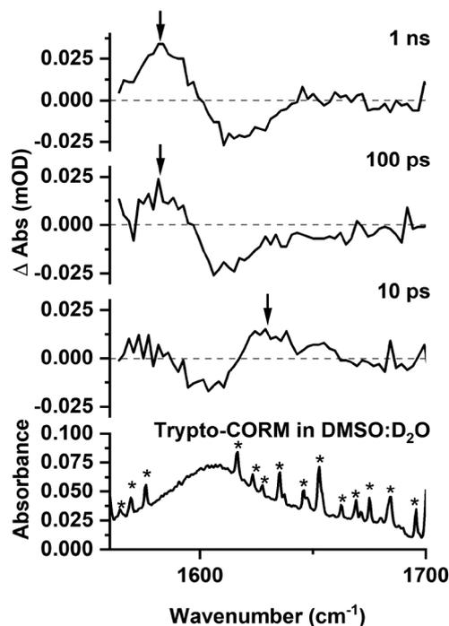
**Fig. 9** Bottom IR spectrum of trypto-CORM in DMSO:D<sub>2</sub>O (1:9 v:v) in the region 1560–1700 cm<sup>-1</sup>. Top time-resolved difference IR spectra for the photolysis (400 nm) of trypto-CORM in NCMe with pump–probe delays of 10 ps, 100 ps, and 1 ns, band positions marked with an arrow. \* indicates bands due to H<sub>2</sub>O contamination.
