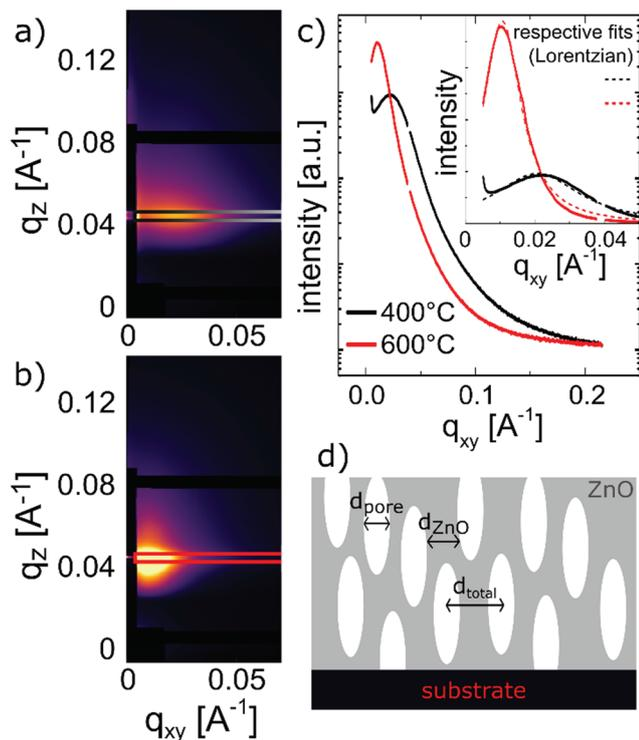
**Fig. 6** GISAXS measurement of the MLD-derived ZnO layers calcined at (a) 400 °C and (b) 600 °C; (c) interference peaks and their fitting with Lorentzian functions in order to extract the peak width  $\delta$ ; (d) a sketch of the extracted distances in the porous structures after calcination.
