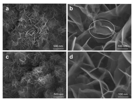
Fig. 3 (a) and (b) SEM images of 10-cycle ALD MnO $_x$  nano-islands grown on NiFe-LDH nanosheets, and (c) and (d) the original NiFe-LDH without modification.
