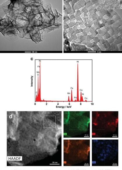
Fig. 4 TEM bright-field micrograph (a), high-resolution (HRTEM) micrograph (b), EDX (c), and HAADF-STEM image and EDX elemental mapping of 10-cycle MnO<sub>x</sub>/LDH (d). The white box in (d) indicates the selected region for the HRTEM micrograph in (b).
