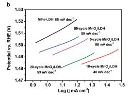
Fig. 2 The cyclic voltammetry curves (a) and Tafel plots (b) of ALD  $\rm MnO_x/NiFe-LDH$  electrodes measured in 1 M KOH (aq) at a scan rate of 1 mV s<sup>-1</sup>.
