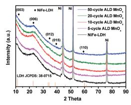
Fig. 1 XRD patterns of NiFe-LDH and with 5 cycles, 10 cycles, 20 cycles, and 50 cycles of ALD  $MnO_x$  grown over NiFe-LDH catalysts.
