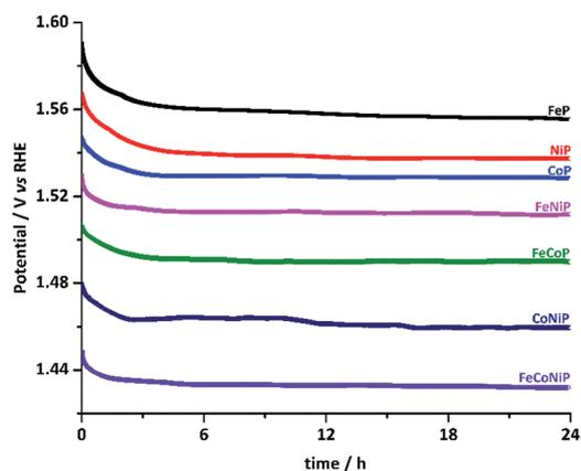
Fig. 4 Chronopotentiometric curves for TMP pre-catalysts recorded at a constant current density of 10 mA cm<sup>-2</sup>.
