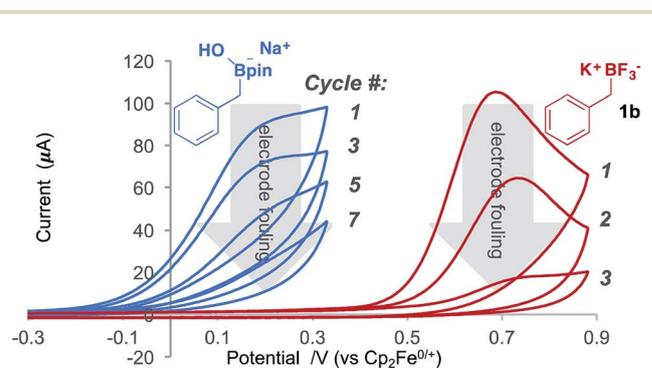
Fig. 3 Cycled CVs reveal a current loss due to benzylic radical grafting and subsequent electrode fouling. CVs of **1a** + NaOH in MeCN and TBAP (0.1 M) and oxo-TEMPO (5 mM) (blue) and **1b** (5 mM) with dihydroanthracene (5 mM) in MeCN and TBAP (0.1 M) (red).
