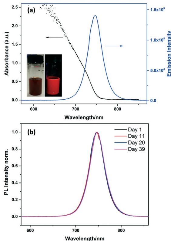
Fig. 3 (a) Absorption and photoluminescence of MAPbI<sub>3</sub> NCs solution in toluene. The insets show the solution under ambient and UV light. (b) PL spectra taken for MAPbI<sub>3</sub> NCs solution over 39 days. The solution was stored in a sealed vial at room temperature in the dark.
