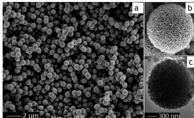
Fig. 2 SEM (a and b) and TEM (c) images of the TiO<sub>2</sub> spheres.
