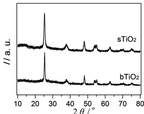
Fig. 1 XRD spectra of the as-prepared sTiO<sub>2</sub> and bTiO<sub>2</sub>.
