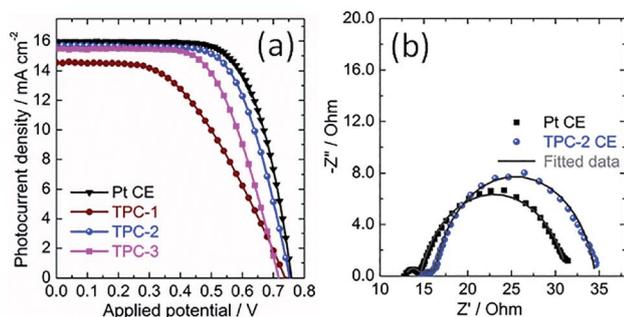
Fig. 6 (a) Characteristic photocurrent density–voltage curves of the DSCs with TPC CEs of different thicknesses and Pt CE, measured under solar simulator illumination of 100  $\text{mW cm}^{-2}$  (AM 1.5G); (b) electrochemical impedance spectra of DSCs using TPC-2 and Pt CEs measured under light irradiation, at open-circuit voltage; dots present experimental results, and solid lines show fitted results.
