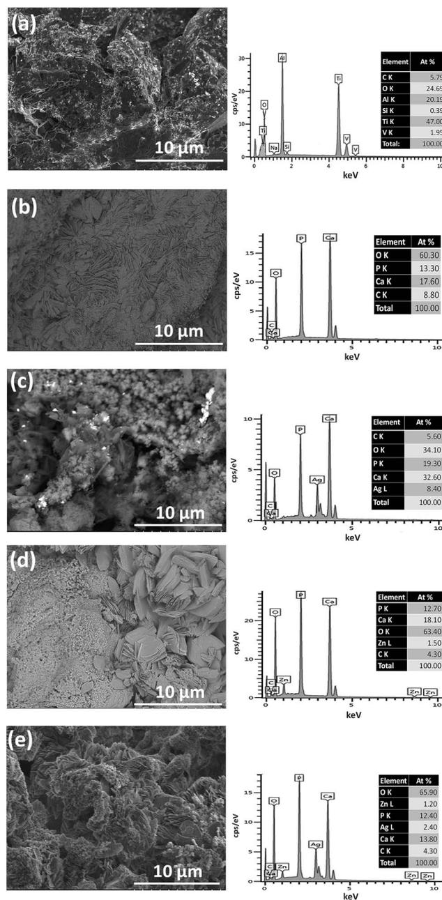
Fig. 10 SEM and the corresponding EDX measurements on the Ti–6Al–4V substrate (a) on a CaP coating (b), on a Ag\_CaP coating (c), on a Zn\_CaP coating (d) as well as on a AgZn\_CaP coating (e). Reprinted with permission from ref. 149 (Copyright © 2016, Elsevier).
