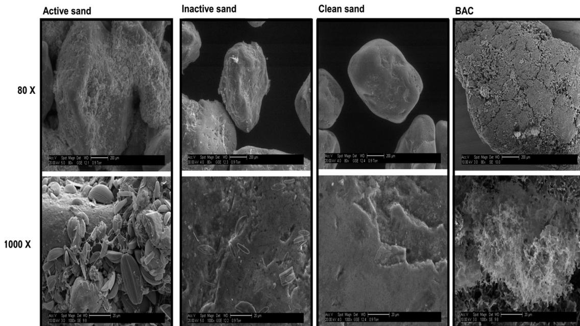
Fig. 1 SEM images of different media at 80 $\times$  (top) and 1000 $\times$  (bottom) magnification. From left to right, active sand, inactive sand, clean sand and biological activated carbon. Scale bars are 200  $\mu\text{m}$  for 80 $\times$  and 20  $\mu\text{m}$  for 1000 $\times$ .
