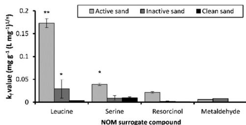
Fig. 3 Comparison of Freundlich isotherm constants ( $k_f$ ) for leucine, serine, resorcinol and metaldehyde in active sand, inactive sand and clean sand. \*\* =  $p < 0.001$ , \* =  $p < 0.05$ ; error bars represent  $\pm 1$  standard deviation.
