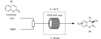
Continuous flow trifluoromethylation using Langlois reagent.
