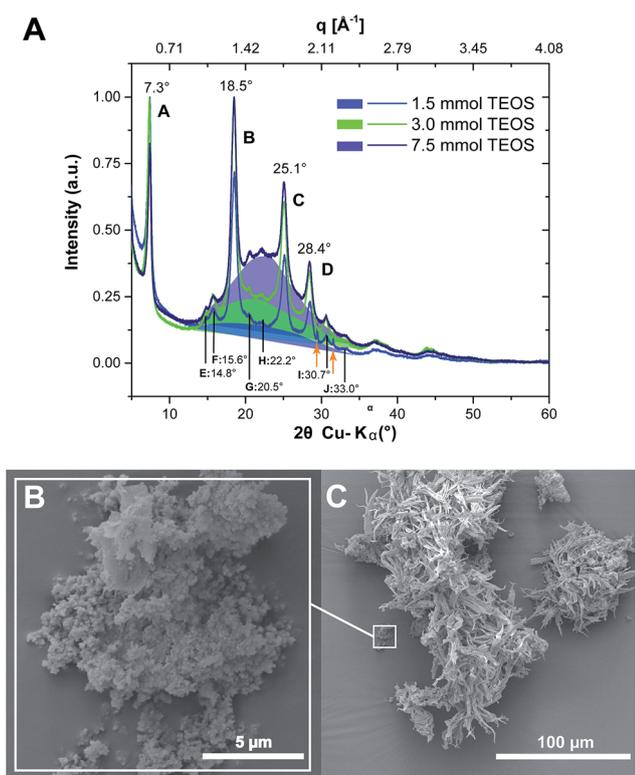
**Fig. 5** PI6/SiO<sub>2</sub> hybrids prepared from HMDA, PMA and TEOS. (A) Diffractograms of PI6/SiO<sub>2</sub> prepared using different  $n_{TEOS}$ ; amorphous backgrounds are highlighted. (B) and (C) SEM images of PI6/SiO<sub>2</sub> at  $n_{TEOS} = 1.5$  mmol; SiO<sub>2</sub> nanoparticles (B) coexist with PI6 ribbons (C).
