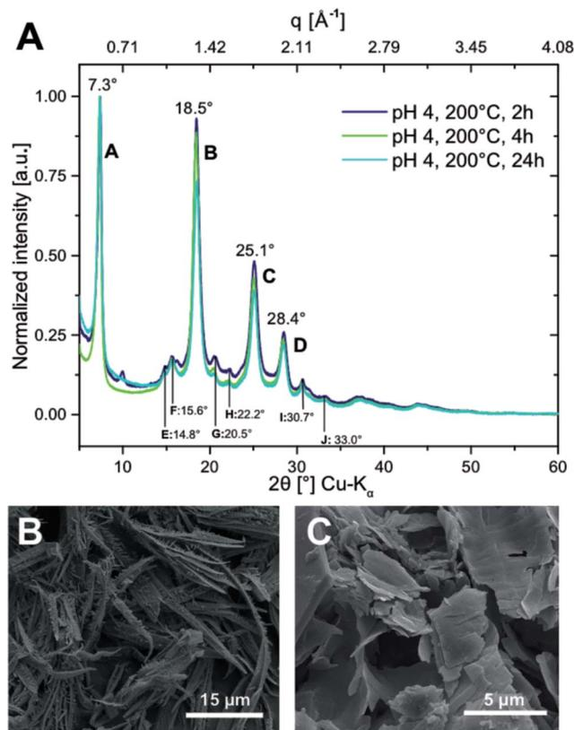
Fig. 3 Crystallinity of hydrothermally prepared PI6. (A) PXRD pattern of PI6 prepared at  $200^\circ\text{C}$  and pH = 4 at  $t_{\text{R}} = 2 \text{ h}$  (dark blue); 4 h (green) and 24 h (turquoise). Reflections are labelled (A)–(J) with annotated scattering angles  $2\theta$  (Cu-K $\alpha$ ). (B) SEM image of PI6 synthesized at  $200^\circ\text{C}$  and pH = 4 for 24 h. (C) SEM image of PI6 synthesized at  $200^\circ\text{C}$  and pH = 1 for 24 h.
