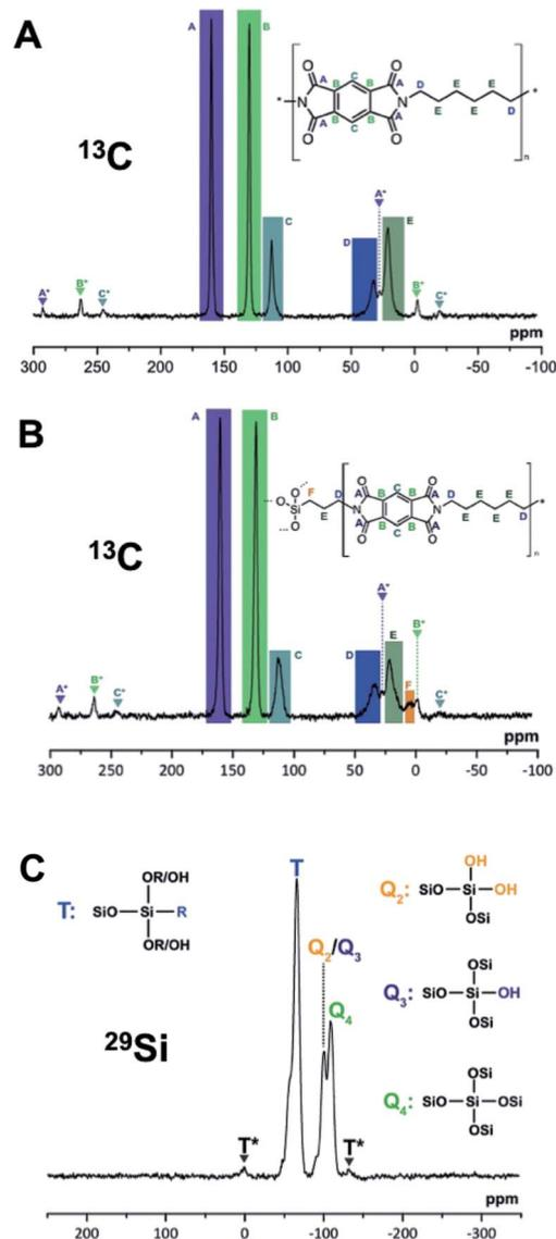
Fig. 8 Solid-state MAS NMR spectra. Spinning side-bands are labelled with \*. (A) <sup>13</sup>C spectrum of PI6 after sintering. (B) <sup>13</sup>C spectrum of PI6/SiO<sub>2</sub> after sintering. (C) <sup>29</sup>Si spectrum of PI6/SiO<sub>2</sub> after sintering.
