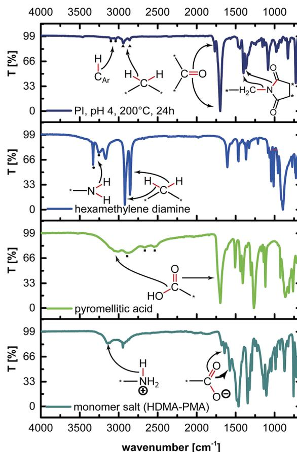
Fig. 2 ATR-FTIR spectra of PI6 and monomers. From top to bottom: PI6, HMDA, PMA, and monomer salt. Mode assignments are illustrated by molecule drawings.
