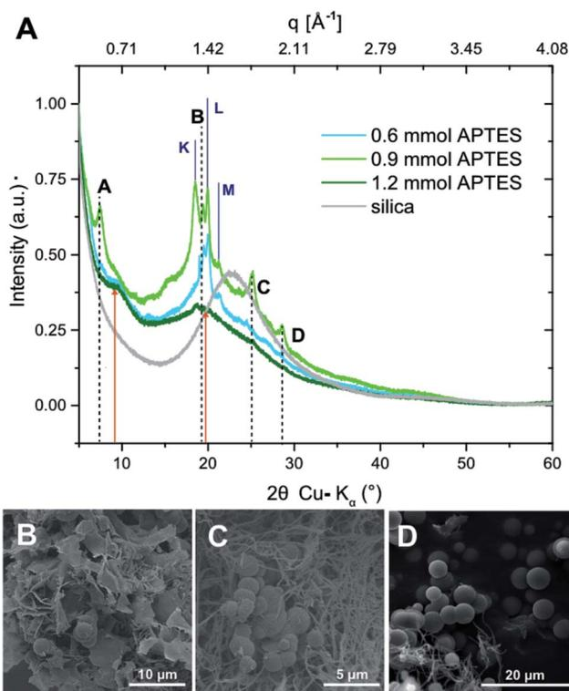
Fig. 6 PI6/SiO<sub>2</sub> prepared from PMA, HMDA, APTES and TEOS. (A) Diffractograms of the hybrids prepared at different  $n_{\text{APTES}}$ , and diffractogram of hydrothermally synthesized SiO<sub>2</sub> for comparison (grey). (B)–(D) SEM images of the corresponding hybrids at  $n_{\text{APTES}} = 0.6$  mmol (B),  $n_{\text{APTES}} = 0.9$  mmol, and  $n_{\text{APTES}} = 1.2$  mmol.
