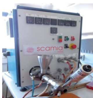
Fig. 7 Representation of a single-screw extruder.
