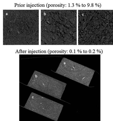
Fig. 6 Possible decrease of the porosity in polycaprolactone reinforced with natural hemp fibers after an injection process (porosity measured by scanning electron microscopy and image analysis).
