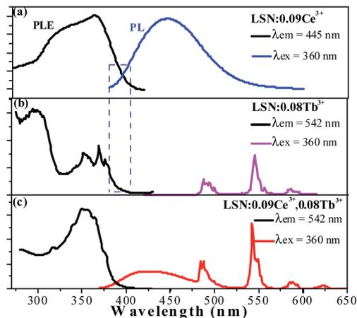
Fig. 5 The PL and PLE spectra of the as-synthesized LSN:0.09Ce<sup>3+</sup> phosphor (a), LSN:0.08Tb<sup>3+</sup> (b), and LSN:0.09Ce<sup>3+</sup>,0.08Tb<sup>3+</sup> (c).
