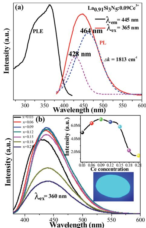
**Fig. 4** (a) PL and PLE spectra of the as-synthesized LSN:0.09Ce<sup>3+</sup> phosphor; (b) the emission spectra of LSN:*x*Ce<sup>3+</sup> with different Ce<sup>3+</sup> contents. The inset above shows PL intensity of the LSN:Ce<sup>3+</sup> samples as a function of the Ce<sup>3+</sup> concentration and the inset below shows the photograph of the LSN:0.09Ce<sup>3+</sup> phosphor under 365 nm excitation.
