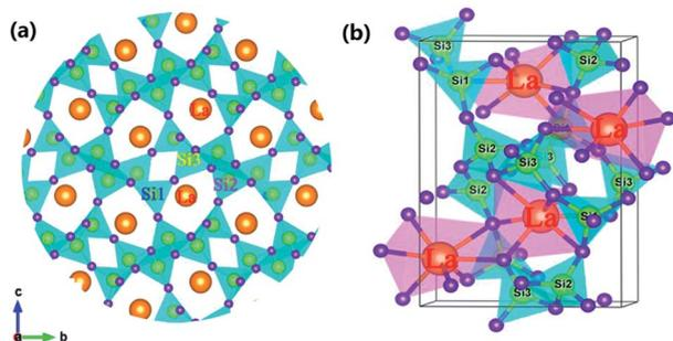
**Fig. 3** (a) Crystal structure of LaSi<sub>3</sub>N<sub>5</sub> along *a*-axis direction. The orange, yellow and purple represent the La, Si and N atoms, respectively. (b) The same coordination environment of La atoms.
