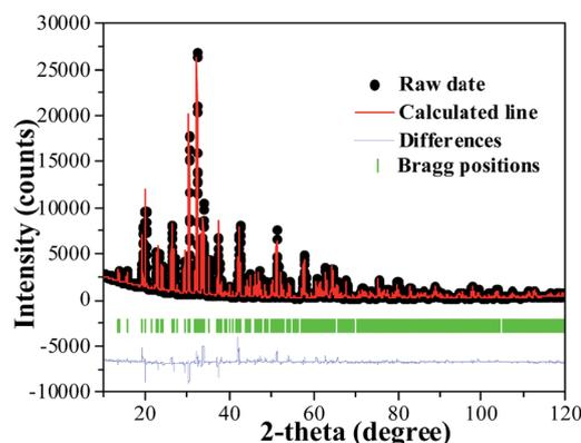
Fig. 2 Rietveld refinement of the XRD pattern of LaSi<sub>3</sub>N<sub>5</sub>. Bragg reflections are indicated with green tick marks.
