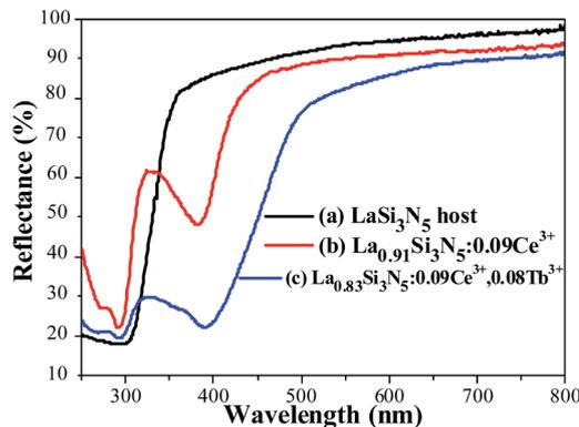
Fig. 6 Reflectance spectra of LaSi<sub>3</sub>N<sub>5</sub> host (a), La<sub>0.91</sub>Si<sub>3</sub>N<sub>5</sub>:0.09Ce<sup>3+</sup> (b), and La<sub>0.83</sub>Si<sub>3</sub>N<sub>5</sub>:0.09Ce<sup>3+</sup>,0.08Tb<sup>3+</sup> (c).
