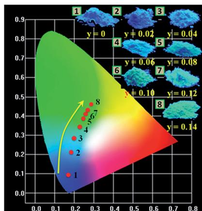
Fig. 11 CIE chromaticity coordinates diagram of LSN:0.09Ce<sup>3+</sup>,yTb<sup>3+</sup> (y = 0, 0.02, 0.04, 0.06, 0.08, 0.10, 0.12, 0.14) (point no. 1–8) and the digital photographs of corresponding samples under 365 nm UV lamp.
