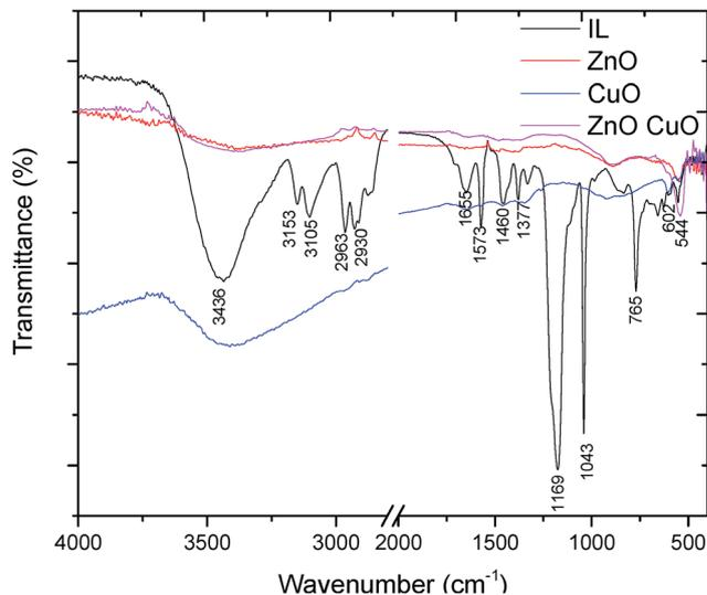
Fig. 4 FT-IR spectrums of the synthesized samples.
