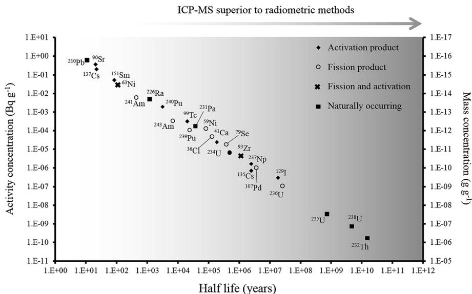
Fig. 1 Half-life versus minimum detectable activity (activity that gives count rate that is  $>3$  times standard deviation of the background count rate) and concentration of selected radionuclides, labelled according to their method of production. Adapted from Russell *et al.* (2014).<sup>1</sup>
