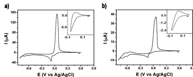
Fig. 3 Cyclic voltammogram of a solution of **1** (a) and **2** (b) ( $2 \times 10^{-4}$  mol  $L^{-1}$ ) in  $NaCH_3COO/H^+$  buffer solution (0.5 M, pH = 4.4). Inset: Cyclic voltammogram of the same solution in a potential range restricted to the first reduction wave observed in the main voltammogram. In both cases, the scan rate was  $5$  mV  $s^{-1}$ , while the working and counter electrodes were glassy carbon and Pt mesh respectively.
