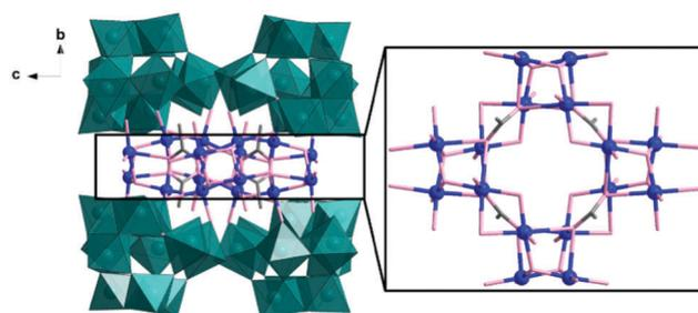
Fig. 1 Representation of the polyanion cluster of 1 (left) and the {Cu<sub>16</sub>} core in the cluster (right). The {W<sub>11</sub>} building units are shown as teal polyhedra, Cu as blue sphere, O and C as rose and grey sticks.
