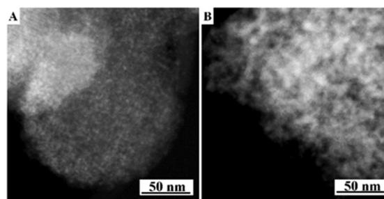
Fig. 3 STEM images of 20 wt% Cu supported AF-MCM-48 (A) and AF- $\gamma$ -Al<sub>2</sub>O<sub>3</sub> (B).
