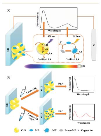
Fig. 1 Schematic illustration of (A) the WR-PEC photocurrent generation process of CdS and MB in a visible light range, and (B) the sensing principle for Cu<sup>2+</sup>
