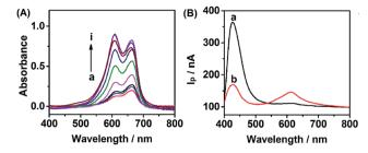
Fig. 4 (A) Absorption spectra of 1 mM leuco-MB aqueous solution incubated with different concentrations of  $Cu^{2+}$  from 0 to 0.1 mM. (B)  $I-\lambda$  curves of CdS modified ITO electrode incubated with 1 mM leuco-MB in the absence (a) and presence (b) of 0.1 mM  $Cu^{2+}$ .
