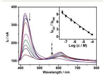
Fig. 6  $I-\lambda$  curves of the optimized WR-PEC sensor in response to different concentrations of Cu<sup>2+</sup>: 0, 40 nM, 100 nM, 0.4, 1.0, 4.0, 10, 40 and 100  $\mu$ M (from a to i). Insert: plot of  $I_{pQD}/I_{pMB}$  vs. the logarithmic value of Cu<sup>2+</sup> concentration.
