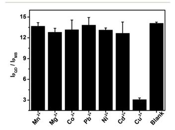
Fig. 7  $I_{pQD}/I_{pMB}$  of the PEC sensor in response to 0.1 mM Mn<sup>2+</sup>, Mg<sup>2+</sup>, Co<sup>2+</sup>, Pb<sup>2+</sup>, Ni<sup>2+</sup>, Cd<sup>2+</sup>, 10  $\mu$ M Cu<sup>2+</sup> and buffer.
