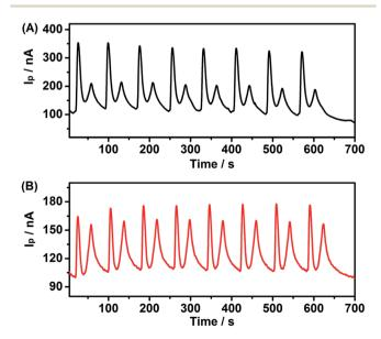
Fig. 8 Continuous PEC experiment of CdS modified ITO electrode incubation with (A) 1 mM MB and (B) 1 mM leuco-MB + 40 μM Cu<sup>2+</sup>.
