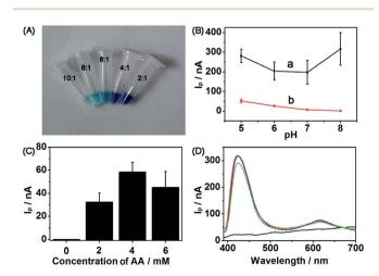
Fig. 5 (A) Photographs of 1 mM MB incubation with AA at different ratios from 10 : 1 to 2 : 1. (B)  $I_{\rm p}$  of CdS (a) and MB (b) at different pHs from 5 to 8. (C)  $I_{\rm pMB}$  at different coreactant concentrations in the detection solution. (D)  $I-\lambda$  curves at the different bias potentials of 0 V (black), 0.1 V (green), 0.15 V (blue) and 0.2 V (red).
