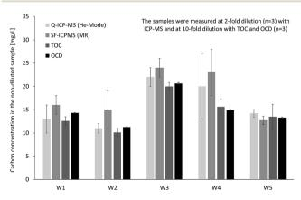
Fig. 3 Determination of total organic carbon in fresh water samples by Q-ICP-MS, SF-ICP-MS, TOC and OCD.
