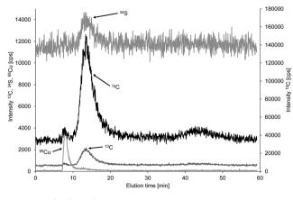
Fig. 7 FFF-Q-ICP-MS fractogram of bovine serum albumin monitoring carbon, sulfur and copper.
