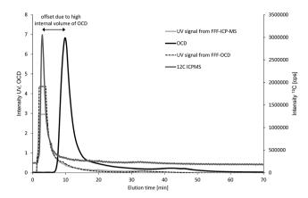
**Fig. 4** Overlay of fractograms of a fresh water sample recorded by FFF-UV-Q-ICP-MS and FFF-UV-OCD. The UV signals suffer from detector overload and were only used for qualitative comparison of the elution profiles from the two FFF systems.
