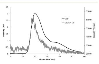
**Fig. 5** Overlay of fractograms of a soil extract recorded by FFF-Q-ICP-MS and FFF-OCD (the offset of 6 minutes between the fraction elution times from OCD and ICP-MS detection due to the larger internal volume of the OCD was determined by flow injection without FFF separation and subtracted from the elution time).
