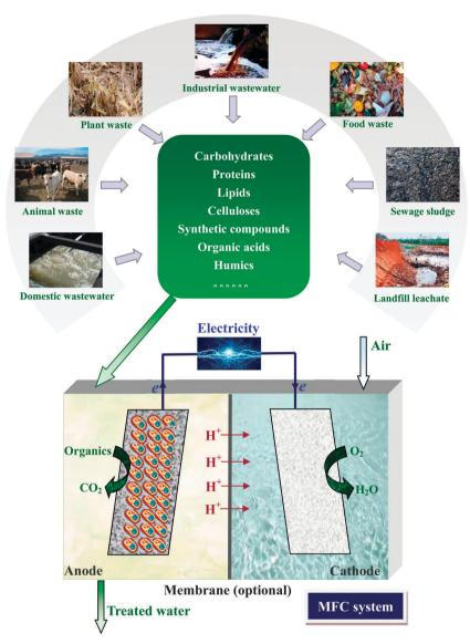
Fig. 1 Electricity generation from wastes by MFC.
