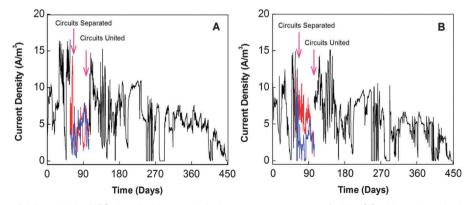
Fig. 10 Current profiles of 4 liter tubular MFCs installed in a municipal wastewater treatment facility: (A) with activated carbon powder as catalyst at cathode; and (B) with both the activated carbon powder and Pt as catalyst at cathode (Reprinted with permission from ref. 149. Copyright 2013 American Chemical Society).
