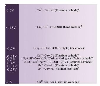
Fig. 16 External voltages applied for the production of various chemicals (data are obtained from ref. 212<sup>a</sup>, 209<sup>b</sup>, 207<sup>c</sup>, 210<sup>d</sup>, 208<sup>e</sup> and 204<sup>f</sup>).
