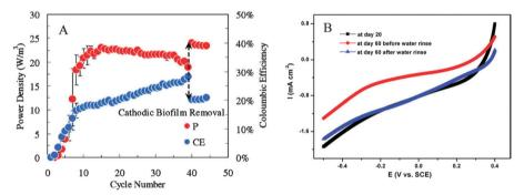
Fig. 12 (A) Power density (P) and coulombic efficiency (CE) of MFC influenced by the growth of cathode biofilm; and (B) linear sweep voltammetry of cathode showing the performance deterioration due to cathode clogging by alkali salts from day 20 to day 60. The current is retrieved after the salt is removed by water rinse (Reprinted with permission from ref. 92 and 164. Copyright 2012 Elsevier Ltd and 2009 American Chemical Society).
