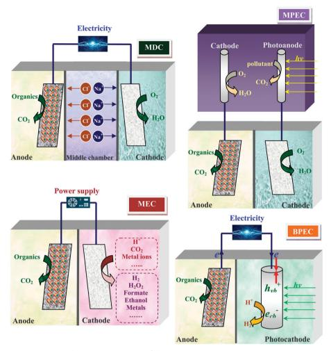
Fig. 15 Principles for the in situ utilization of power generated in MFC for various applications
