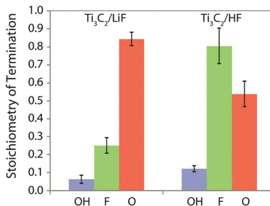
Fig. 3 Composition of the  $\text{Ti}_3\text{C}_2\text{T}_x$  surface functional groups produced by etching of the  $\text{Ti}_3\text{AlC}_2$  in HF and LiF–HCl solutions, per  $\text{Ti}_3\text{C}_2$  formula unit, *i.e.*  $\text{Ti}_3\text{C}_2(\text{OH})_x\text{F}_y\text{O}_z$ .
