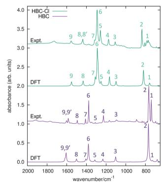
Fig. 7  $\,$  IR absorption spectra of HBC and HBC-Cl. Wavenumbers computed by DFT have been scaled by 0.98.
