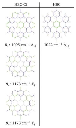
**Fig. 10** Representation of the normal modes of HBC-Cl relevant for Raman spectroscopy in the B region according to DFT calculations.
