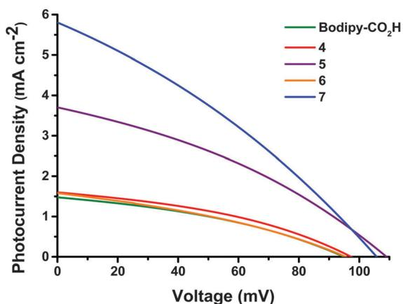
Fig. 3 Current–voltage characteristics of the dye-sensitized NiO solar cells with 0.1 M I<sub>2</sub>, 1.0 M Lil electrolyte and **4** (red), **5** (purple), **6** (orange), **7** (blue) and **Bodipy-CO<sub>2</sub>H** (green) under AM 1.5G (100  $\text{mW cm}^{-2}$ ) illumination.
