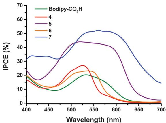
Fig. 4 Comparison of IPCE spectra of the dye-sensitized NiO solar cells with 0.1 M I<sub>2</sub>, 1.0 M Lil electrolyte and **4** (red), **5** (purple), **6** (orange), **7** (blue) and **Bodipy-CO<sub>2</sub>H** (green).
