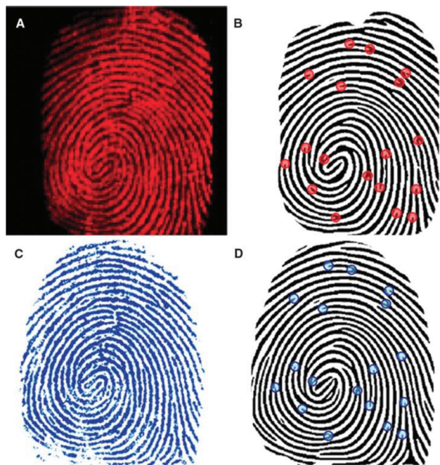
Fig. 3 (a) DESI-MS image of the distribution of cocaine on an LFM blotted on glass. (b) Computer-generated fingerprint from the DESI image. (c) Ink fingerprint blotted on paper and optically scanned. (d) Computer-generated fingerprint from the optical image. Some of the automatically detected points of interest (minutiae) are represented by dots in (b) and (d). 36 Reproduced from ref. 36 with permission from the American Association for the Advancement of Science.
