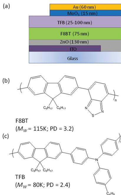
Fig. 3 (a) Schematic illustration showing the device architecture investigated and individual layer thicknesses, (b and c) molecular structures, molecular weight ( $M_w$ ) and polydispersity (PD) information for F8BT and TFB.
