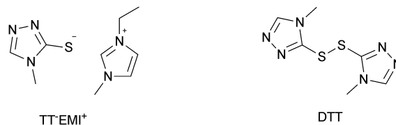
Fig. 13 Structures of the \text{TT}^-\text{EMI}^+ /DTT-based redox couple. Adapted and reprinted from ref. 193.
