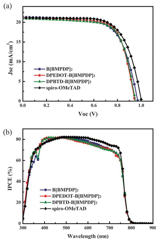
Fig. 3 (a) Photocurrent–voltage ( $J$ – $V$ ) curves of the solar cells with **B[BMPDP]<sub>2</sub>** (■), **DPEDOT-B[BMPDP]<sub>2</sub>** (●), **DPBTD-B[BMPDP]<sub>2</sub>** (▲) and **spiro-OMeTAD** (◆) as the HTMs, respectively. (b) Corresponding IPCE spectra.
