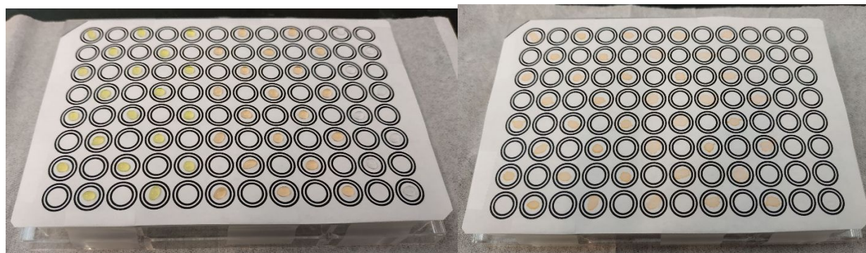
23 24 25 26 27 28 29 30 31 32 33 34 35 Figure 1. A representative experimental set up using a paper plate: columns 1-5: calcein dye (yellow), columns 6- 36 10: [calcein•PAMAM] complex (orange), columns 11-12: HEPES buffer blanks (clear). Left: wet droplets soon after 37 deposition; right: samples after they were allowed to dry. 38
