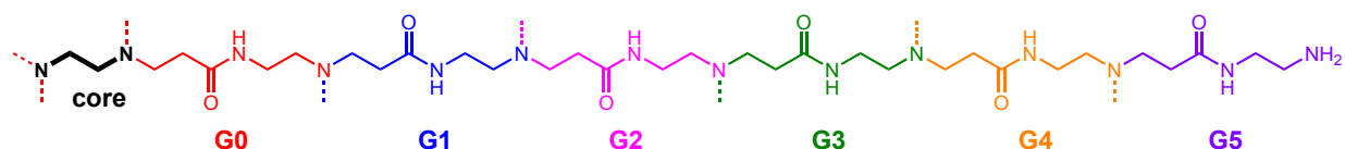
Scheme 1. One branch of a fifth—generation (G5) amine-terminated poly(amidoamine) (PAMAM)dendrimer with an 1,2-diaminoethane core; the dashed lines indicate the position of further branching points along the structure.
