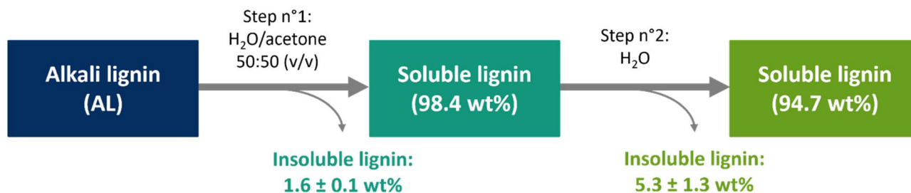
Fig. 1 Schematic representation of the 2-step solubilization process.
