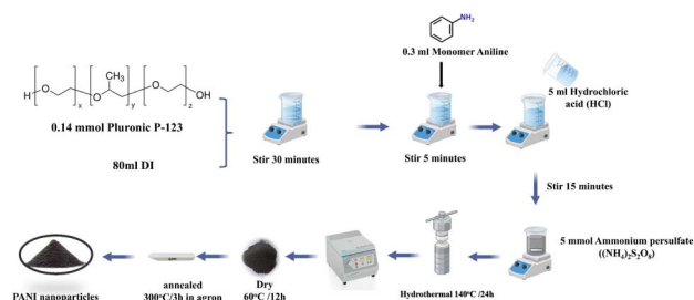
Fig. 10 Process for the hydrothermal synthesis of pure polyaniline (PANI).
