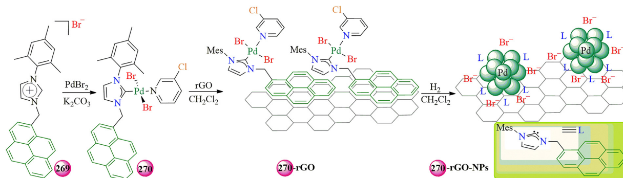
Fig. 75 Bottom-up synthetic procedure of pyrene-tagged palladium nanoparticles immobilized onto graphene. Reproduced with permission from ref. 84 copyright 2023, Elsevier.
